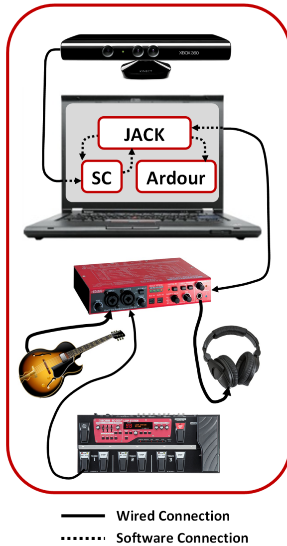
Fig. 8.1: System configuration used throughout participatory design cycle.
