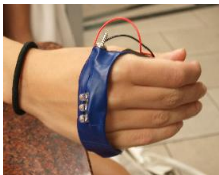
Fig. 3.3: The custom-built sensor strap built for the Videoconferencing Privacy System.
